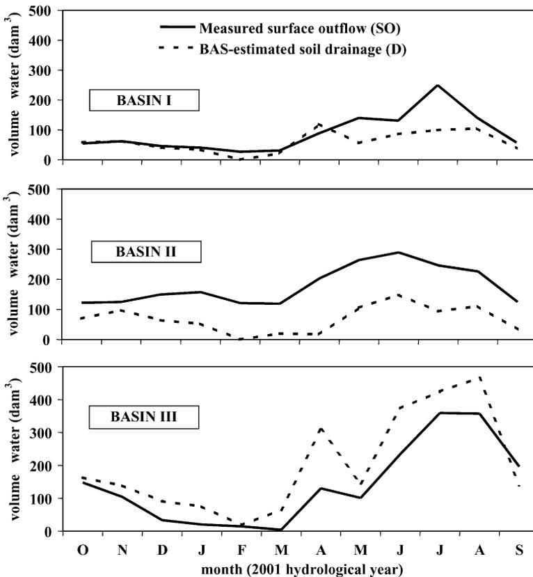
Fig. 4. Monthly measured surface outflows (SO) and BAS-estimated drainage volumes (D) in basins I, II, and III during the 2001 hydrological year.
