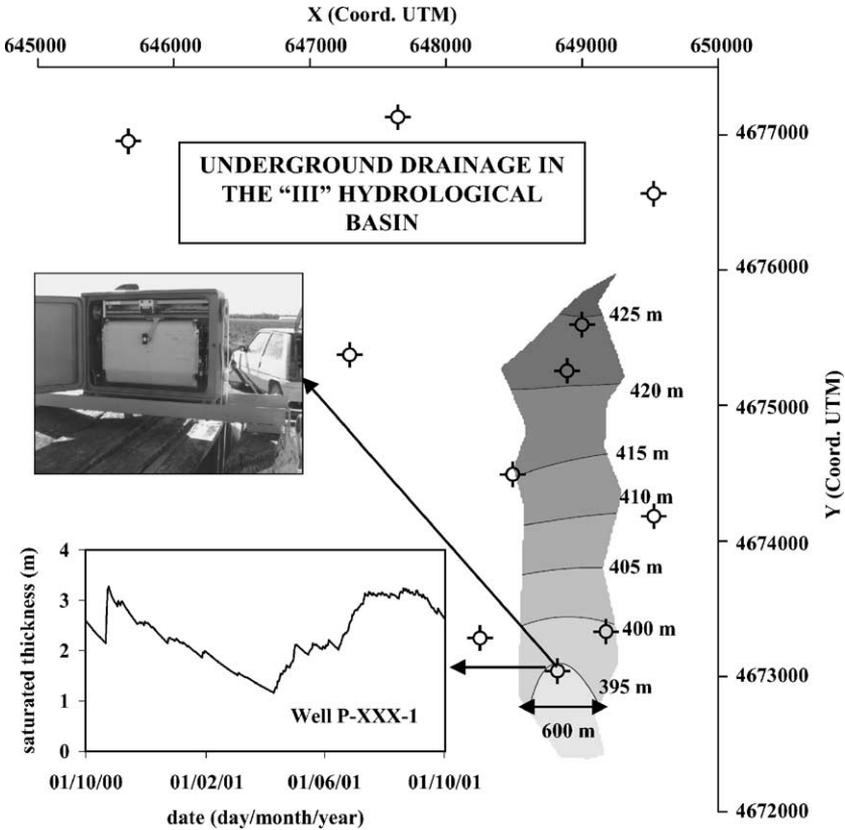
Fig. 3. Isolines map of the mean annual groundwater height estimated in hydrological basin III from the groundwater depths measured every 21 days in 11 wells. The daily saturated thickness of the aquifer measured with a limnigraph at the outlet of basin III during the hydrological year 2001 is also shown.
