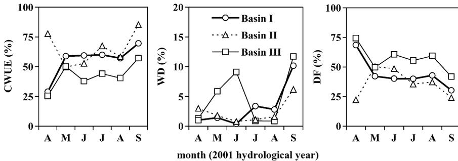
Fig. 5. Monthly consumptive water use efficiency (CWUE), water deficit (WD) and drainage fraction (DF) in the three study basins during the 2001 irrigation season.
