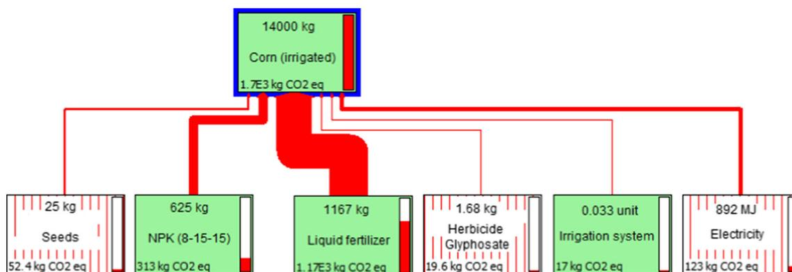
**Fig. 2** Flowchart of annual CO<sub>2</sub> equivalent emissions of irrigated corn grown on 1 ha in the basin of Lerma (Spain). Emissions related to the standard irrigation system are included in the flowchart
